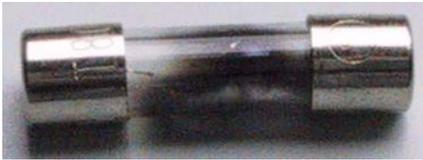
Also a fuse with a value of 3 times the nominal current trips after this test, when a transformer is inside the equipment. Ordinary Inrush current limiters can not react as fast enough of this short voltage dip, and the limiting element stay bridged or hot when a NTC-resistor is used.
